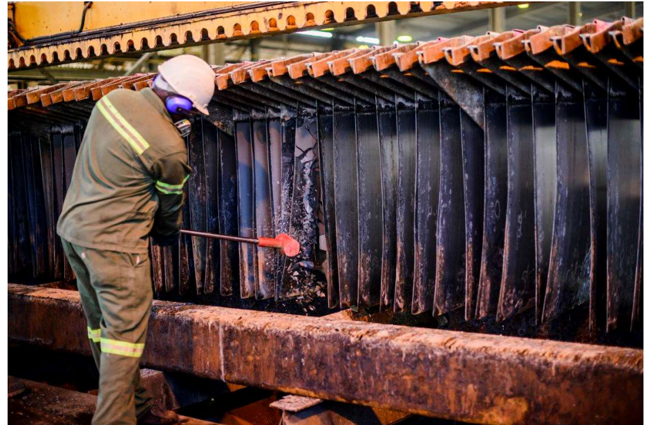
Employees at the Manganese Metal Company use rubber mallets to strip manganese away from steel sheets. The product is then washed and dried before being loaded into bags for export. Manganese Metal Co
